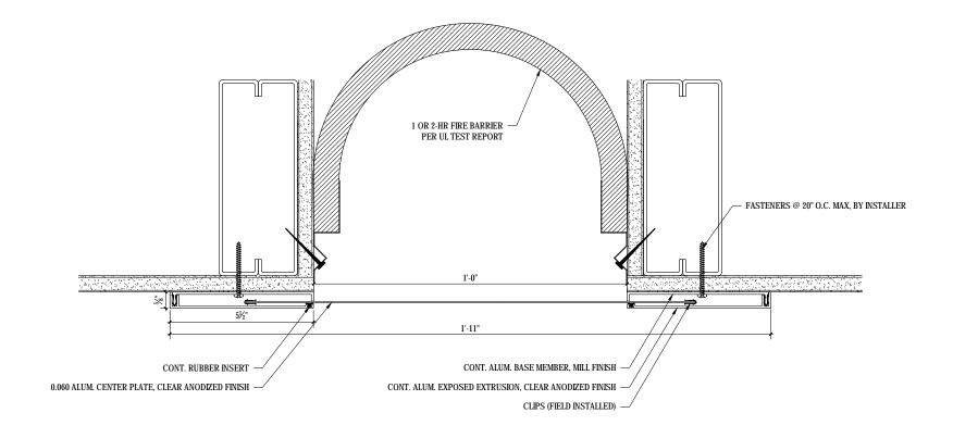
NOTE: 1 HOUR CONSTRUCTION INDICATED 2 LAYERS OF GYPSUM BOARD FOR 2 HOUR CONSTRUCTION
